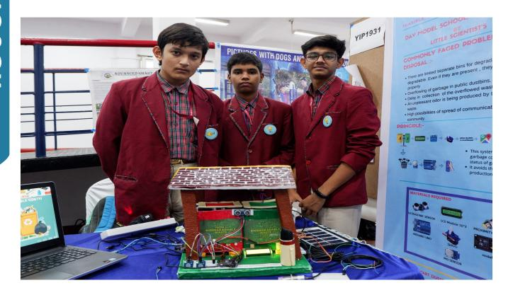
The team came up with a product that helps to keep cities clean, stop garbage bins from overflowing and keep biodegradable and non-biodegradable waste separate. This system helps to monitor the garbage level of the bins and informs garbage collectors to clean the bins via IoT (using nodeMCU), resulting in some quick action that can keep the place clean and hygienic. The bins are also easy to open because of the use of sensors.
