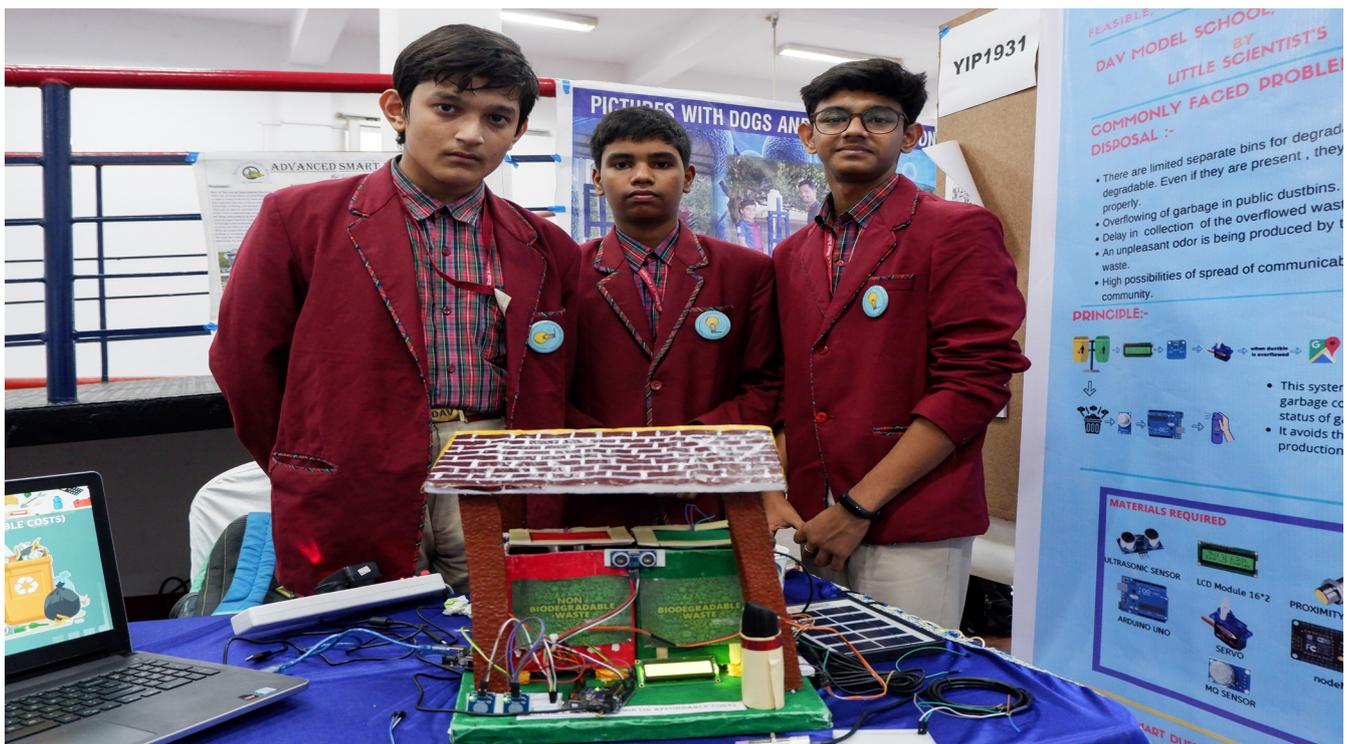
The team came up with a product that helps to keep cities clean, stop garbage bins from overflowing and keep biodegradable and non-biodegradable waste separate. This system helps to monitor the garbage level of the bins and informs garbage collectors to clean the bins via IoT (using nodeMCU), resulting in some quick action that can keep the place clean and hygienic. The bins are also easy to open because of the use of sensors.
