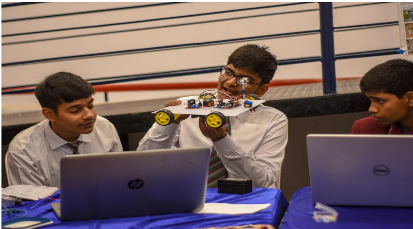
The team came up with an Arduino UNO powered floor cleaner that offers comparable performance for a fraction of the price of commercial floor cleaners. It uses the concept of automated machine learning. This Arduino-based robot can primarily be used in hospitals and other not-for-profit organizations as well as in homes as a cheap alternative to sophisticated floor cleaning appliances which cannot be afforded by everyone.
