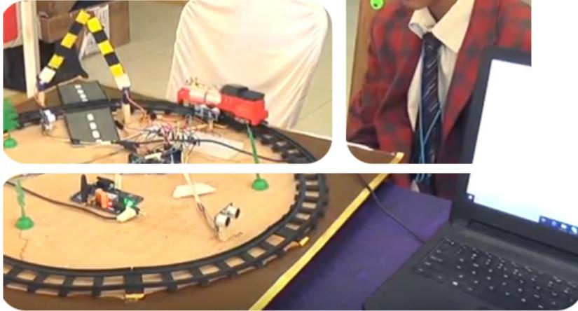
With almost half the total rail accidents taking place at railway crossings, there is a need for a device that removed this flaw. Thus, Team AutoCross came up with a fully automated level crossing system that would eliminate the dangers arising from unmanned level crossings. This simple idea, realized with the help of Arduino IDE, Servo motors and ultrasonic buzzers, can really help in the drastic reduction of mishaps due to negligence.
